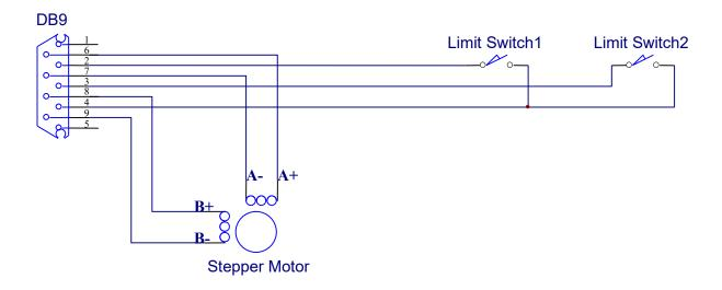
Mechanical Limit Switch 1 is at the opposite end of the stepper motor. It's the home (zero) position.
